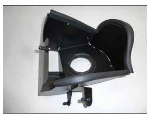
13. Install the heat shield mounting studs onto the heat shield as shown using the provided hardware.
