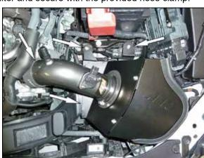
15. Install the complete intake assembly into the vehicle so the mounting studs engage with the factory air filter housing mounts, the intake tube engages the coupling hose and the fresh air intake duct inserts into the heat shield. Align the intake tube and then tighten the hose clamp that secures the intake tube.
