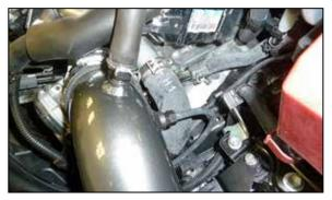
16. Connect the factory vent hoses to the fittings installed into the AEM® intake tube.
