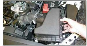
5. Lift up and remove the intake system from the
