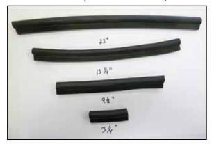
9. Cut the provided edge trim into four sections as shown. 3-1/4", 9-1/2", 13-1/4", 22".
