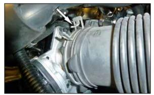
4. Release the spring clamp and disconnect the intake hose from the throttle body.
